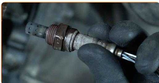
**7** Rengør oxygen sensorens montagested. Brug WD-40 spray.
