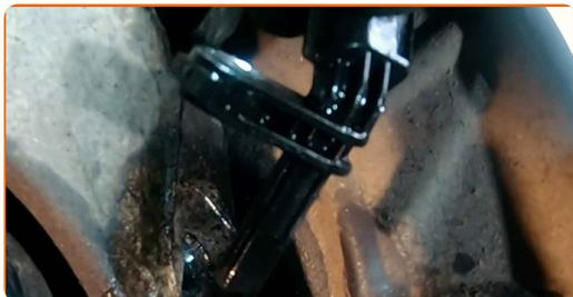
10 Rengør ABS sensorens montagested. Brug en stålbørste. Brug WD-40 spray.
