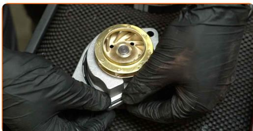
**59** Installer den nye vandpumpe. (Install the new water pump)
