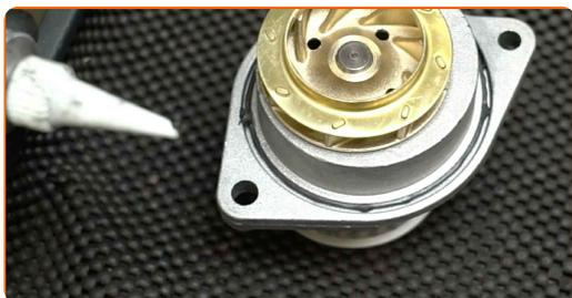
**58** Installer vandpumpe pakningen. (Install the water pump gasket)
