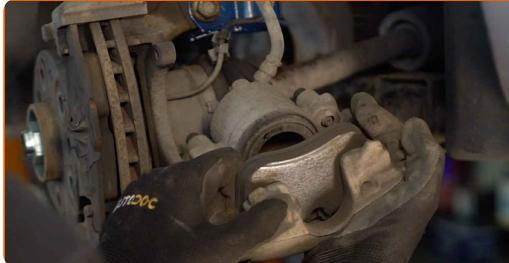
Udskiftning: bremseklodser – VAUXHALL Astra Mk VI (J) (P10) Hatchback.
