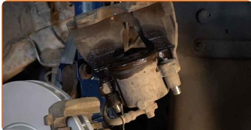
Udkiftning: bremseklodser – VAUXHALL Astra Mk VI (J) (P10) Hatchback.
