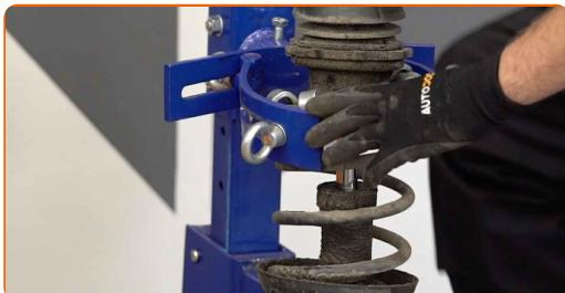
**Udskiftning: fjederben – VAUXHALL Corsa Mk III (D) Hatchback (S07).**
