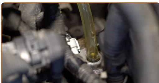
Udskiftning: manuel gearkasseolie – VAUXHALL Corsavan Mk III (D) (S07).
